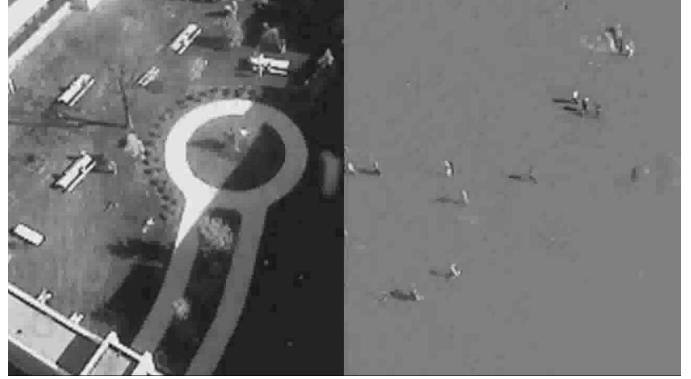
Fig. 2: Close-up of example frame showing results of (left) background, B(x, y, t) , and (right) foreground, F(x, y, t) , separation via RoSuRe-DSP.
