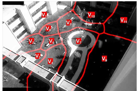
Fig. 3: Region boundaries produced from local maxima of D
